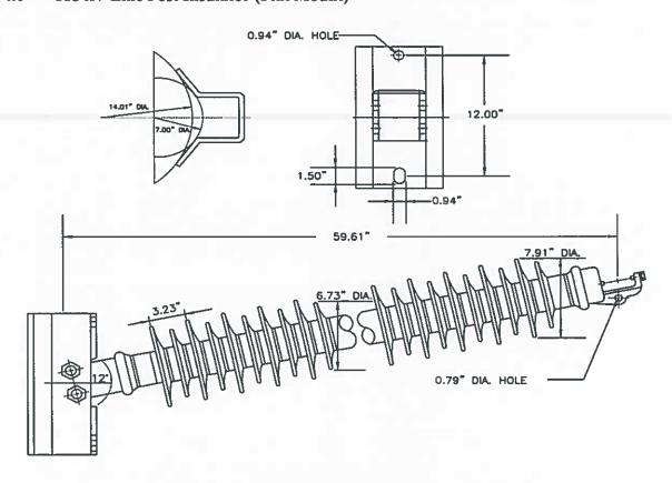
INDEX NO. SSOI0716 (Victor Insulator HP-70DD-1514-3820-XX or equivalent)
