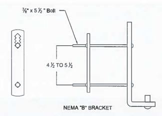
NOTE: NEMA B Bracket must be furnished with all Load Break and Non-Load Break cutouts.
