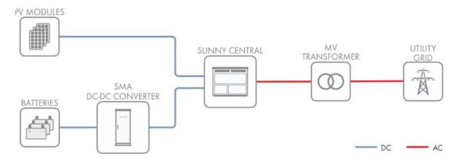
Unfortunately, we didn't see the utility-scale DC-coupled configuration which PV Modules DC-coupled to the BESS Batteries, the BESS Batteries connected to the PCS (instead of PV Inverter), and then connected to the grid. Between PV Modules and BESS Batteries, there should be specific equipment such as Charge Controller for DC-coupling and controls of PV-BESS.
