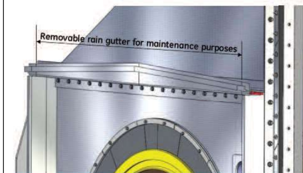
Figure 45. The CHROEM designs offered by GE have a removable rain gutter for ease of maintenance.
