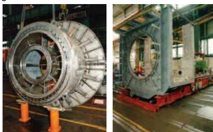
Figure 25. Advanced CHROEM PG6581B aft diffuser has increased dimensions.
