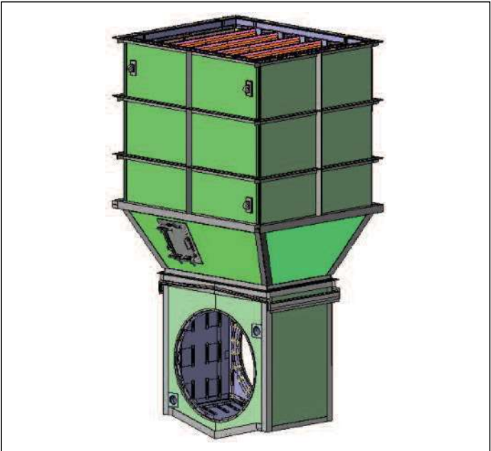
Figure 51. Frame 5 exhaust stack with silencers shown positioned above a vertical split plenum.
