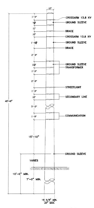
45 FOOT CONCRETE POLE (CLASS A SELF-SUPPORTING)
